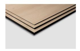
EGGER Compact Laminates are compact laminate according to EN 438. They have a multilayer structure and consist of melamine resin impregnated decorative paper and multiple layers of soda kraft paper impregnated with phenolic resins, which are laminated under high pressure and heat.
